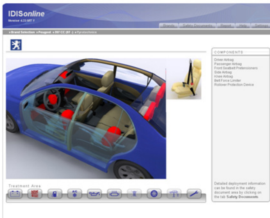
Figure 5 – Pyrotechnic devices in a vehicle
